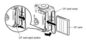
Captured images are recorded on the CompactFlash (CF) card. Make sure that the camera is turned off before inserting or removing the CF card (optional). When no card is inserted, the images are recorded in the camera's built-in memory (11MB).
